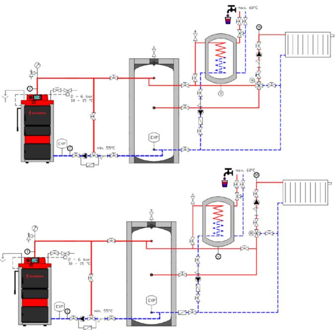
IT IS POSSIBLE TO USE THE PUMP SYSTEM WITH THE THERMOSTATIC VALVE TO PROTECT THE RETURN WATER FROM CH.
