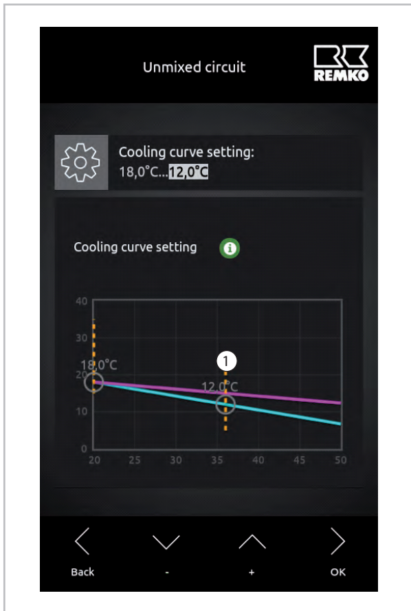
Fig. 14: Setting the outside temperature
